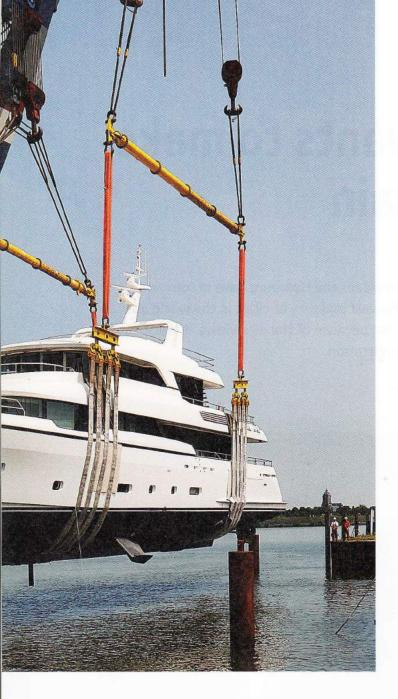
The 36-metre superyacht is the first to feature a hull made of high tensile steel. The innovative use of high tensile steel ensures that the yacht is lightweight, which increases speed further and reduces draft considerably. This makes the yacht ideal for sailing in the Caribbean, especially shallow drafts places like the Bahama's. Because of the features of the high-tensile steel hull, *Brigadoon* will also be fuel efficient.
