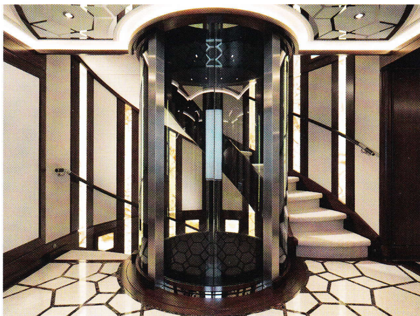
circular glass lift, right, is a dramatic feature. The lift shaft was built outside the boat and lowered into place
