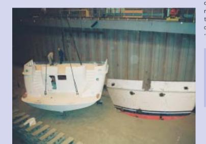
'Rio Rita' was refitted, one couldn't see where the old part ends and the new begins," Alblas adds smiling. A good design of the swimming platform at the new stern was necessary so the yacht would keep good performance at seas rolling in from behind. Also the extra length should not be of negative influence towards the manoeuvrability. The result of the hull extension is that 'Rio Rita' goes faster and makes shorter turns.
