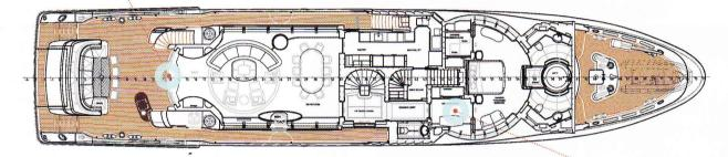
STORAGE: The large tender is out of view until an overhead crane mounted on frames helps it clear the fold-out swim platform. PRIVACY: The full-beam master stateroom is accessed through the office and a short corridor and looks out over the sea.
