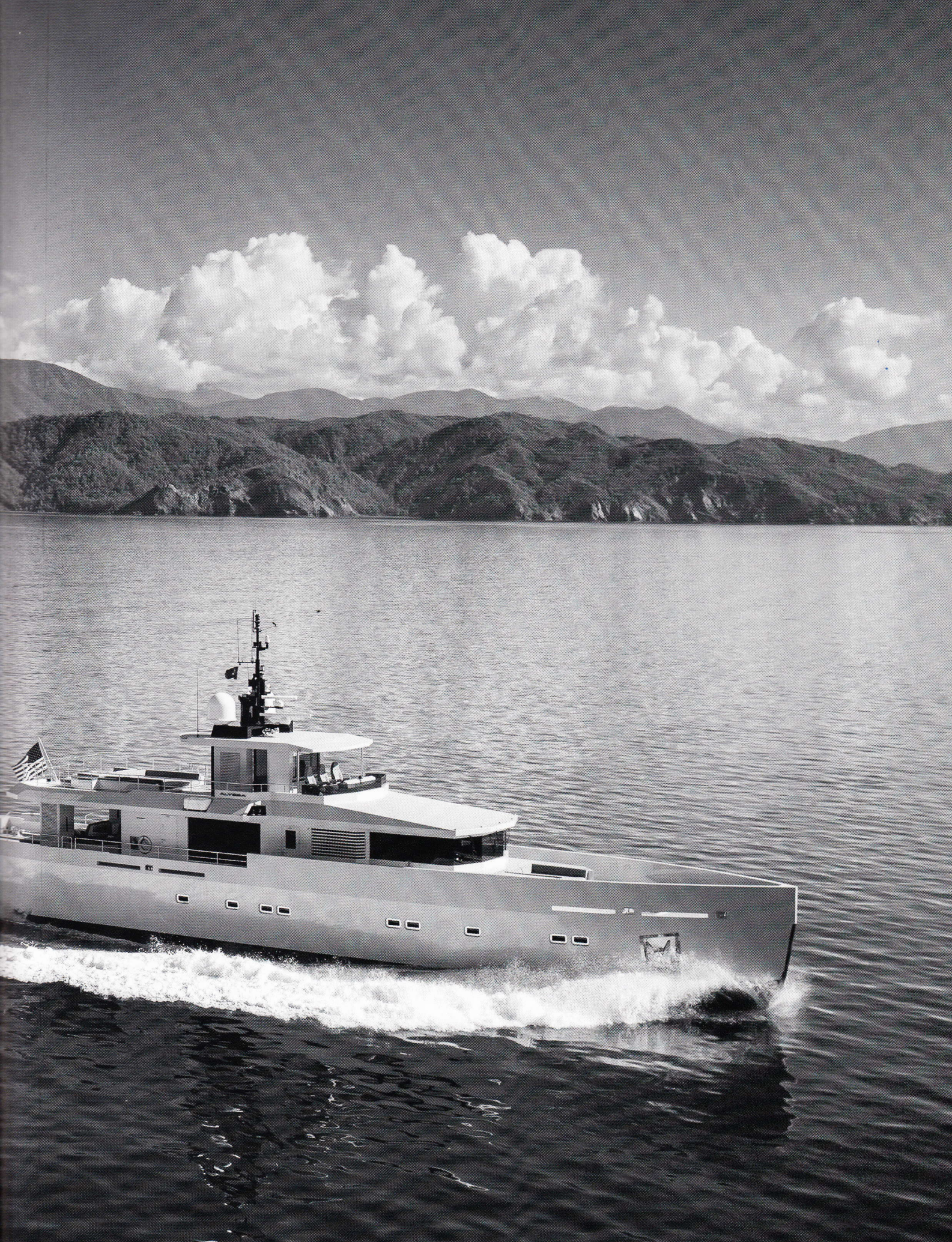
platform he had used on 33.9m Only Now and, with twin Caterpillar C32 1,900bhp engines, that gives Alyssa a cruising speed of 18 knots and a top speed of 21 knots
