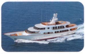
She can store 60000 liter of fuel and 12000 liter of water on board and still get a range of 5,000 nm @ 10 knots. With a maximum speed of 14 knots she will be suitable for blue water cruising around the world.
