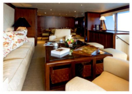
The ceilings were covered with Majilite Destiny Parchment, with a padded backing to reduce noise, and the carpet was also laid on Cloud 9 underlay to reduce noise and vibration. Modern systems were installed within the new joinery, resulting in very comfortable and light cabins.
