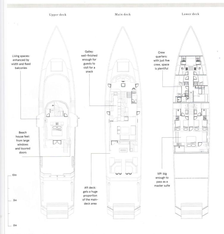
LOA 37.92m Beam 7.4m Draught 1.82m Displacement 172.4 tonnes
